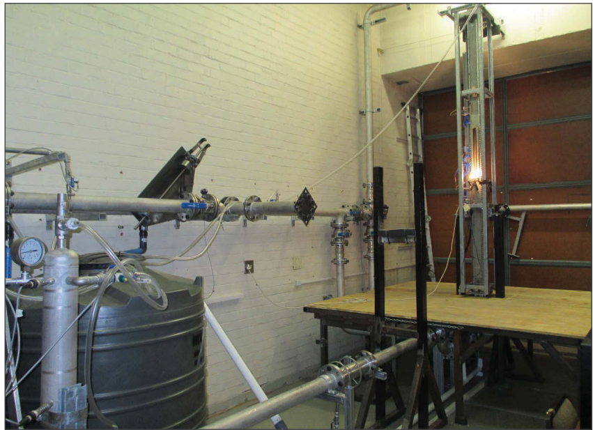
→ The flow loop for testing heated fuel pins.
