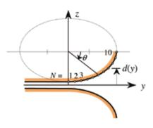
$\rightarrow$  8. Elliptic plate separation profile. Combined with the near-optimal impedance taper, all that is needed is a function to calculate the width from the impedance.
