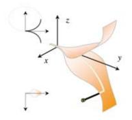
→ 9. TEM horn with elliptical plate seperation and microstrip impedance approximation.
