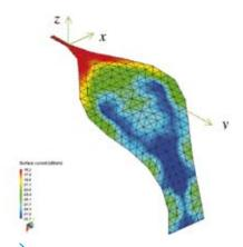
$\rightarrow$  10. Current density on the outside of horn plate surface. Only one plate is shown.
