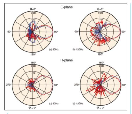
$\rightarrow$  15. Comparison of measured and calculated E-plane ((a) and (b)) and H-plane ((c) and (d)) at 8GHz ((a) and (c)) and 12 GHz ((b) and (d)) for the extreme bandwith horn.
