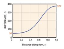
$\rightarrow$  7. Variation of impedance according to the near-optimal impedance function by Hecken<sup>7</sup>.
