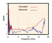
$\rightarrow$  13. Calculated and measured values of the Voltage Standing Wave Ratio vs frequency for the extreme performance horn.
