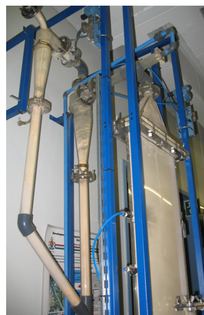
→ Catalyst circulation above the dense bed section.
