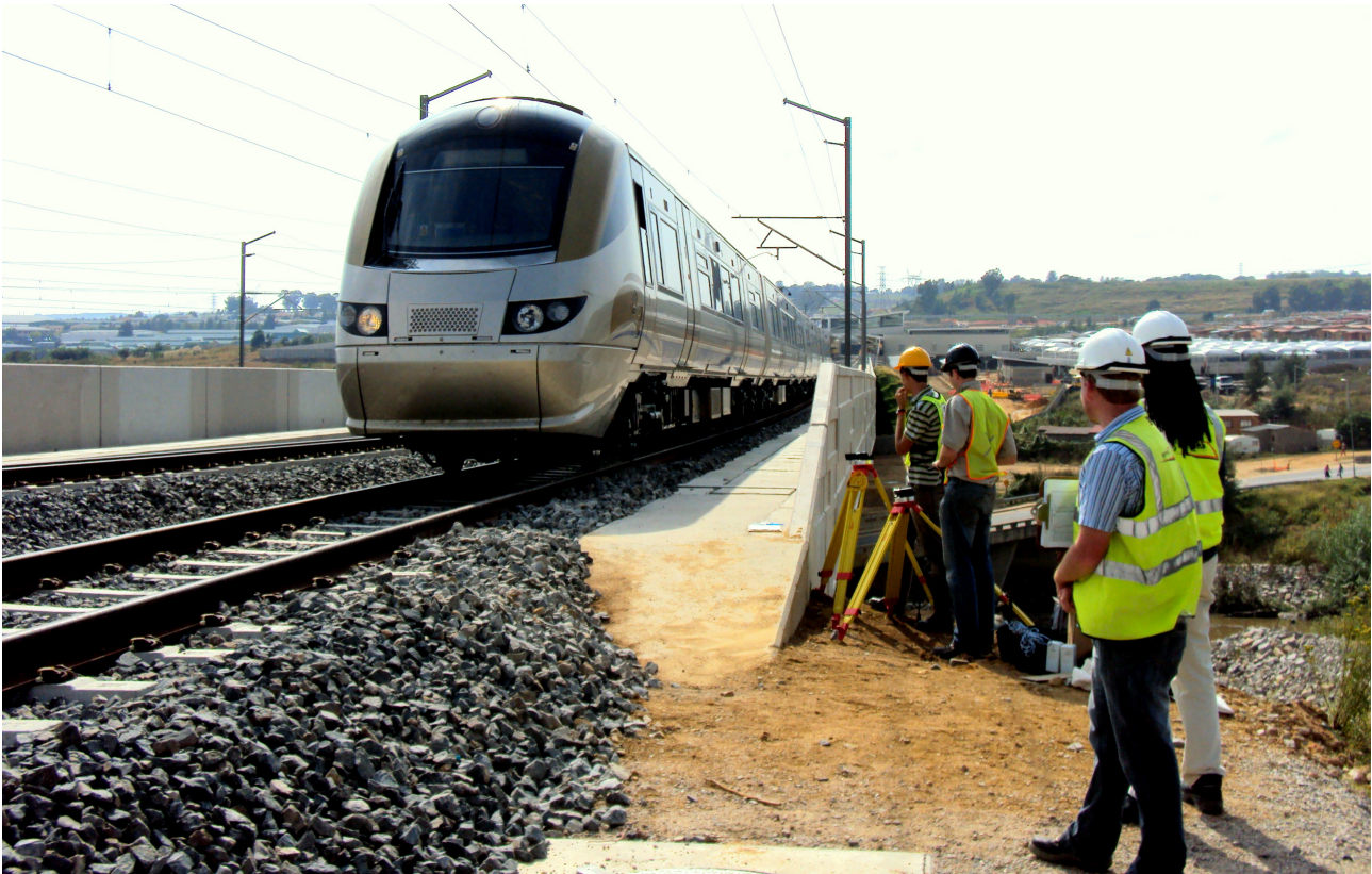
→ Students and staff carry out track performance tests outside Marlboro station on the Gautrain rapid rail link.
