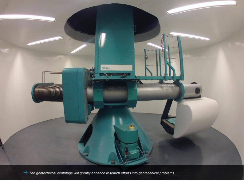
The back analysis of the settlement that was measured during these trials was a complex undertaking that required many assumptions to be made. The behaviour of the surcharge loads will now be modelled in the geotechnical centrifuge, which will entail settlement and soil compressibilities being measured and compared. This may have important applications for future projects when construction has to be carried out on dolomitic soils.
