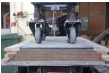
UTCRC centrifuge: A scale model of a section of a Ultra Thin Continuously Reinforced Concrete Pavement (UTCRC) with a scaled heavy vehicle load.
