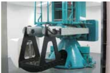
Centrifuge: The Department houses the largest civil engineering centrifuge in the southern hemisphere, accelerating scale models to investigate the behaviour of complex geotechnical problems such as the formation of sinkholes.
