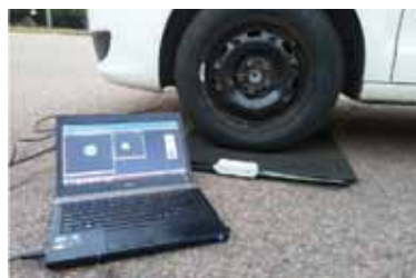
Tyre pressure: Research on the effect of tyre pressure on the stress distribution under vehicle tyres.
