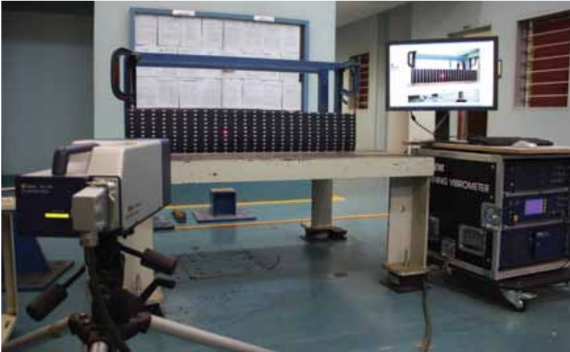
→ Figure 2. Scanning laser vibrometer measurements on a composite model aircraft wing.
