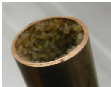
FIGURE 3.12: SAND ROUGHENED TUBE
