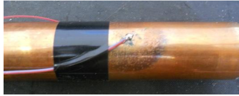
FIGURE 3.16: THERMOCOUPLES ATTACHED TO TUBE
