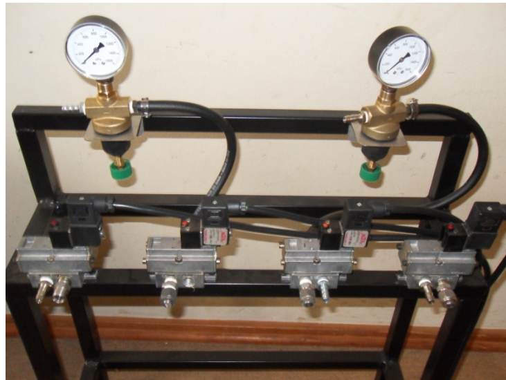
Figure 3.2 Main Frame With Valves Installed
