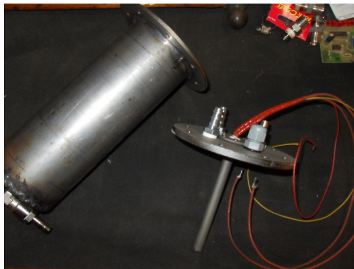
Figure 3.1 Test Capsule With Heater Installed
