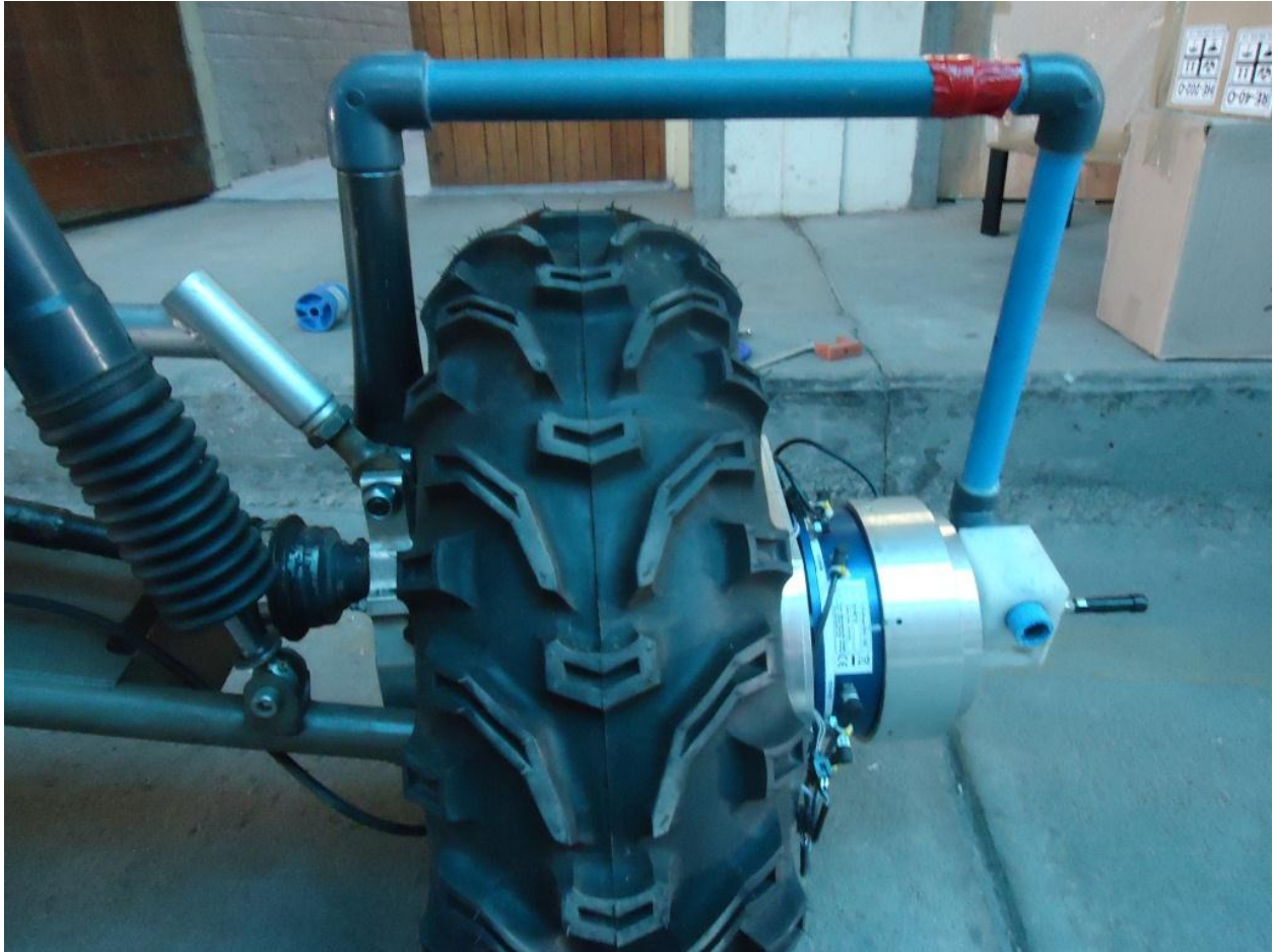
Figure 34: Wheel force transducer with the telemetry and angular positioning equipment
