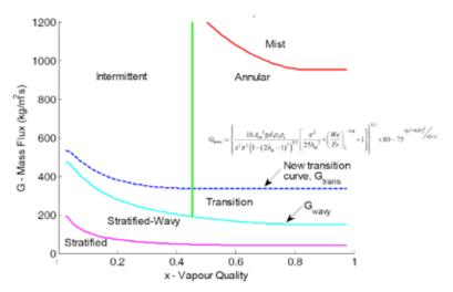
$\Rightarrow$  New flow pattern transition criterion ( $G_{trans'}$  blue dashed line in figure) developed by Ridhwaan Suliman as part of his final year undergraduate project. This new criterion differs significantly from that which is currently used by designers of two-phase flow heat exchanger systems.
