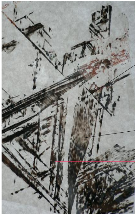
Figure 3. A lattice excitation that starts from an atomic cascade. It looks something like a shock wave but contains an unexplained inner structure.
