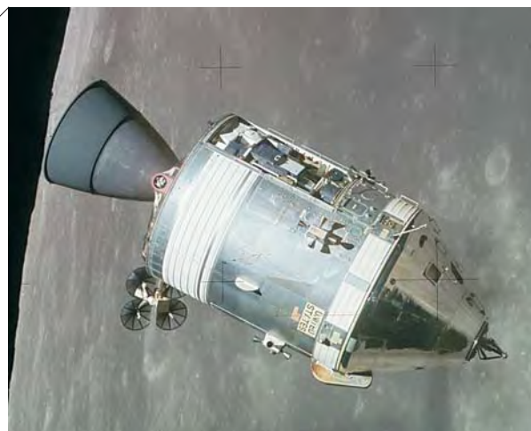
The black rocket nozzle of Apollo 15 is made from niobium-titanium alloy.
