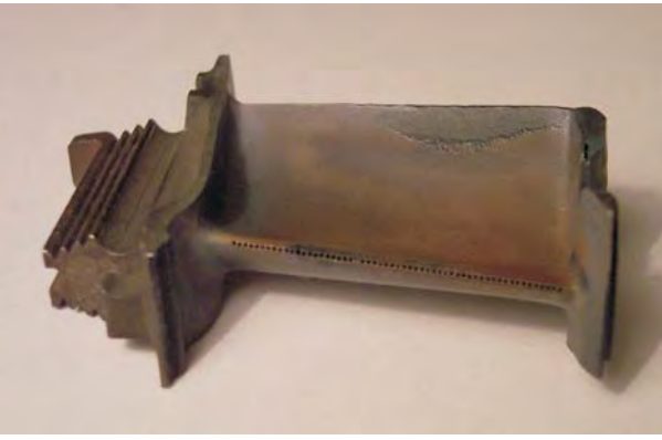
Jet engine turbine blade from nickel superalloy
