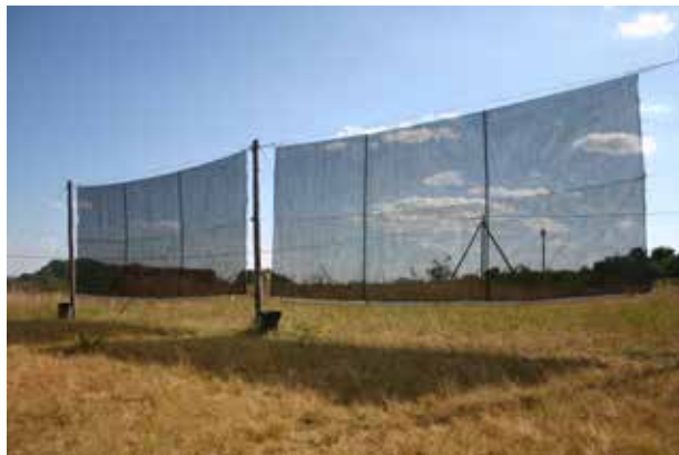
Fog net at Tshiavha Primary School. This fog net was erected by second year meteorology students in 2007.
