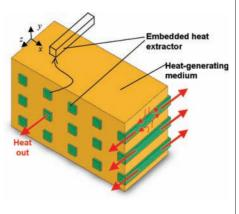
→ Schematic representations of embedded heat extraction insert schemes indicating the aided flow of heat to the environment.
