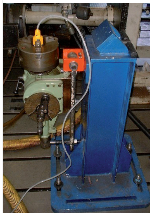
→ Testing equipment for investigating the effects of geophone misalignment in the Sasol Laboratories at the University of Pretoria. The geophone is the bright yellow object in the top centre-left of the photograph. The apparatus is used to shake the geophone assembly with vibrational frequencies similar to those measured in the mines, and to determine the fidelity of the geophone record with the machine-input frequency. In this way, the effect of geophone misalignment can be determined and compensation to reduce it implemented.
