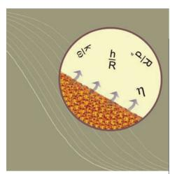
→ A cross-section of a rotary kiln shows the particles rolling down the surface of the bed, enhancing evaporation or gas-solid reaction as the kiln turns clockwise. The rate (designated as efficiency,  $\mu$ ) depends only on k/w (ratio of reaction rate to rotation speed) and  $h/\sum$ (bed fill) for low rates and an additional third parameter R/d<sub>p</sub> (kiln radius/particles diameter) for fast processes.
